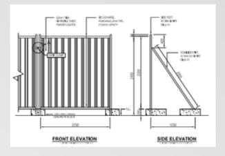
Fencing sheet -Size: Generally 2m. width x 2m. height (other sheet sizes can be made on order). Overall height - 2.2m
